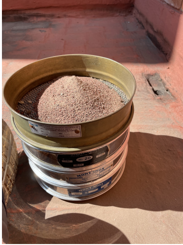
Figure 3: Sieves used to separate samples
