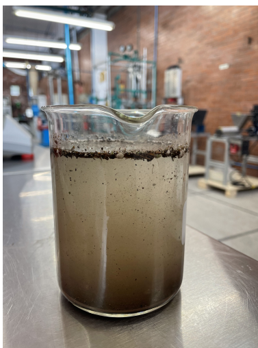
Figure 2: Precipitation as a method to separate organic matter in the sample
