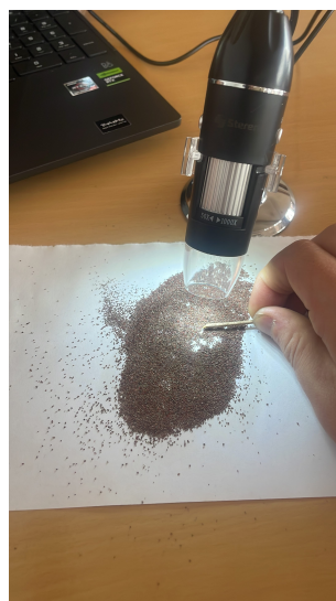
Figure 8: Sample analysis using an optical microscope with USB connection
